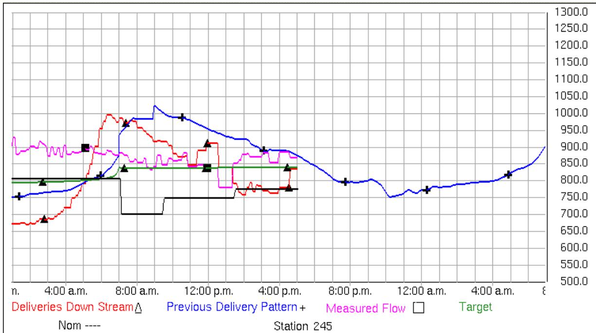
Generally during the day the Measured-Flow should be less than the Deliveries-Down-Stream because load drops off at night. We should be drawing on linepack during the day. G2 will issue a warning under Recommendations if linepack is being drawn too low, ie. G2 thinks that you will not be able to build the linepack up during the evening.
