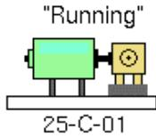
if the status of 25-C-01 = "Running" and the discharge-pressure-1 of sta-25 < the maximum-discharge-pressure of sta-25 - 20 and the rpm of 25-c-01 < 750 and 25-engine-run >= 4 and the throughput-1 of
